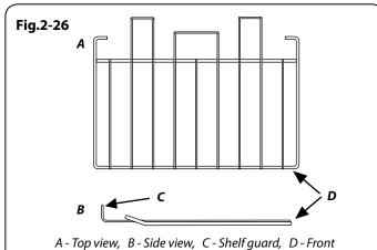
The shelf guard should be at the back pointing upwards
